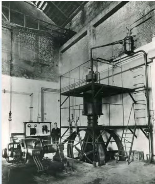
First experimental plant for the production of synthetic ammonia designed by Giacomo Fauser. September 21 st , 1921
